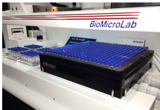
The thermal rack contains 378 2mL vials.
