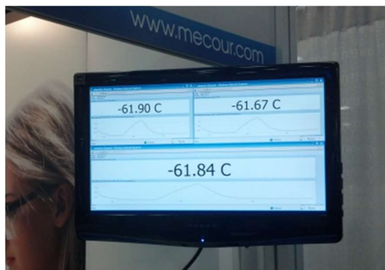
System provides real-time feedback and uniform temperature for all sample vials. During SLAS 2015, the system maintained a real time uniform temperature of -65°C for all vials. (MéCour offers systems running as low as -90°C.)
